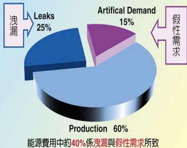
Typical Compressed Air Consumption
