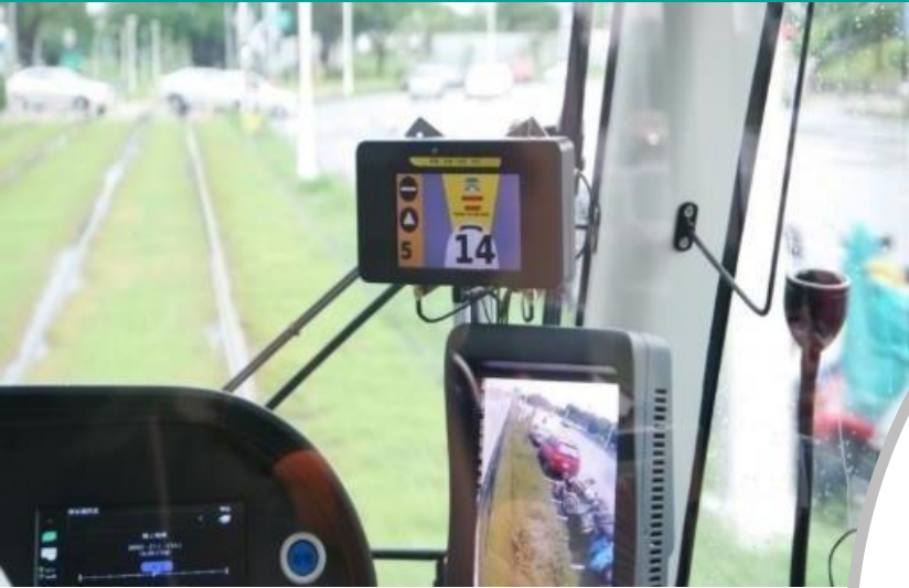
Light rail train's anti-collision system
