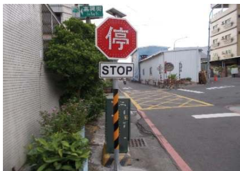
The solar-powered stop sign for all driving directions at the intersection of Jiasing Street and Benchang Lane, Cinghua Street in Niaosong District
