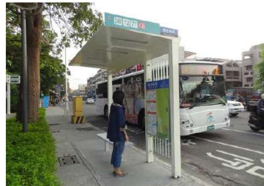
A cantilever style bus waiting shelter
