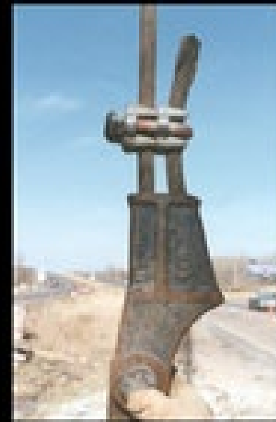
Double Grip, Double Saddle Wire Rope Clamp (Two Separate Saddles with U-Bolt)
