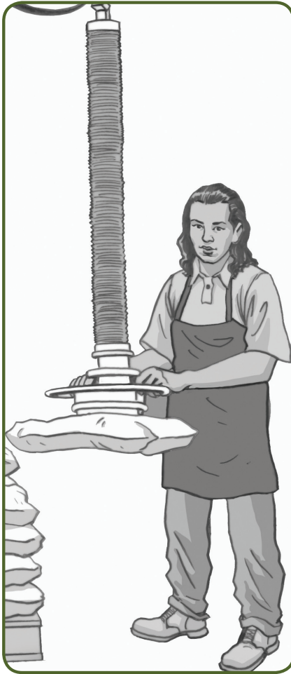
Figure: An employee operating a pneumatic lift and moving device. More details on Page 11, Figure 9.
